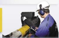
The A4910 - Lubri is designate for lubrication replenishment process. During this process the instrument measures the actual lubrication of a bearing and tells the operator when the amount of lubricant is ideal. So it is ensured that we do not under or over lubricate. The instrument enables you to make the whole lubricating process simpler, and decrease lubricant costs and machine maintenance costs.
